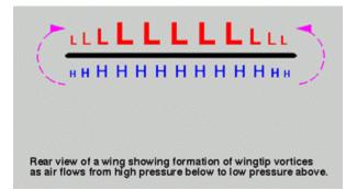
The most effective way to minimize induced drag is to increase span, as induced drag is inversely proportional to the span squared. Highly efficient airplanes like gliders have very high span for the amount of lift they are producing. Winglets are a way to create the effect of higher span without actually increasing the physical span. They are useful when there is an artificial constraint on wingspan (like a draft limitation on a keel).
