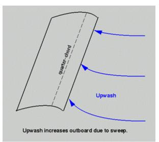
Sweep has the effect of increasing the upwash on the outboard wing sections. As a wing is angled aft, flow over the outboard sections must pass by the low pressure on top of the wing sections immediately inboard and forward. The close proximity of that low pressure to the air just outboard causes the outboard flow to turn upward more, resulting in higher upwash on the outboard wing.
